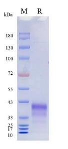
On SDS-PAGE under reducing (R) condition. The gel was stained overnight with Coomassie Blue. The purity of the protein is greater than 90%.
